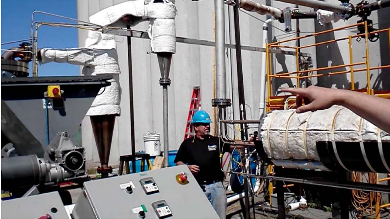
Figure 5 Modified Capstone microturbine operating completely on syngas directly from the biomass gasifier
