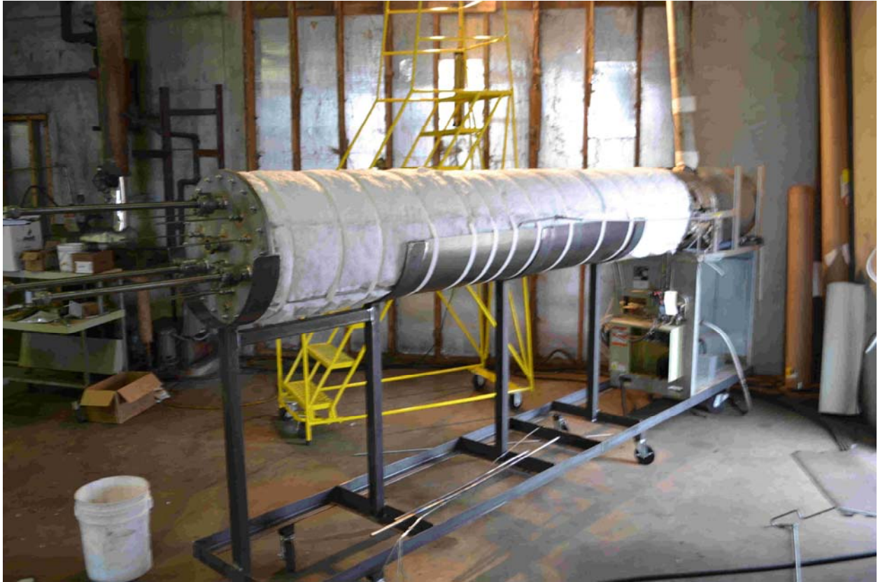
Figure 3 Image of indirectly heated microturbine
